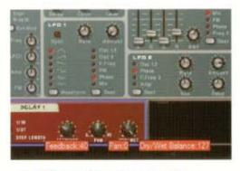
Feedback button controls how much delay is repeated, so the longer the feedback level, the longer it takes for the delay to decay. The Dry/Wet knob controls the amount of processed sound fed to the Aux buss.
