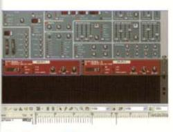
Stereo delay: By adding a second DDL-1 Line to your mixer and assigning it to the Aux 2 buss, you can create a neat stereo delay. Just set the Pan of either unit to hard left or right — you now have the basis of a stereo delay. Use two different delay times to get a chiming effect.
